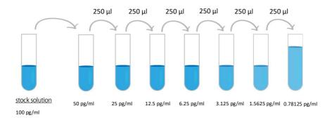
Dilute EPO Receptor standard as according to the table below:
