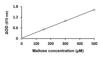
ARG82180 Maltose Assay Kit (Colorimetric) typical data demonstration image
